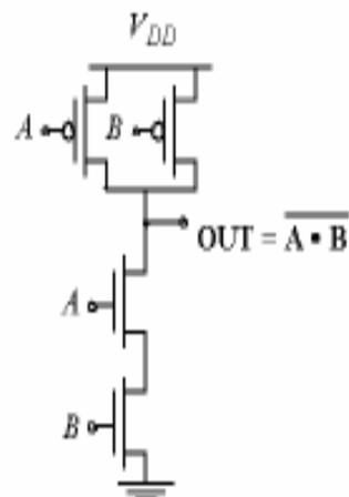
PDN:  $G = A \cdot B \Rightarrow$  Conduction to GND
