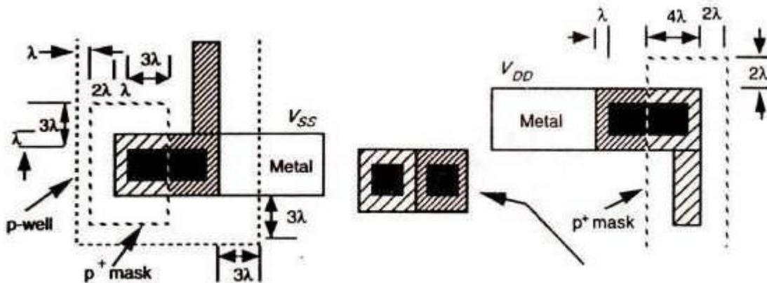
From the above diagram it is also clear that split contacts may also be made with separate cuts.
