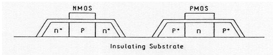
The SOI CMOS process is considerably more costly than the standard p & n-well CMOS process. Yet the improvements of device performance and the absence of latch-up problems can justify its use, especially for deep-sub-micron devices.
