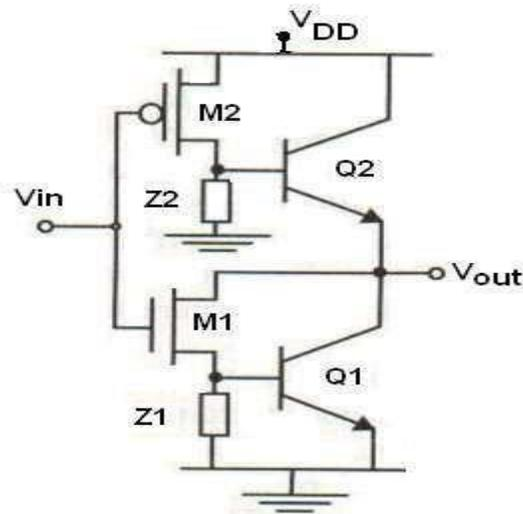
When input,  $V_{in}$ , is high ( $V_{DD}$ ), the NMOS transistor ( $M1$ ), turns on, causing  $Q1$  to conduct, while  $M2$  and  $Q2$  are off, as shown in figure (b). Hence, a low (GND) voltage is translated to the output  $V_{out}$ . On the other hand, when the input is low, the  $M2$  and  $Q2$  turns on, while  $M1$  and  $Q1$  turns off, resulting to a high output level at the output as shown in Fig.(b).
