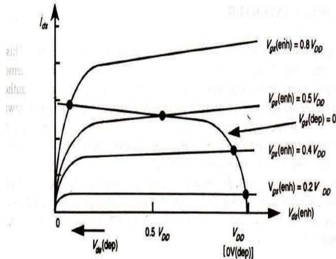
From the graph it is clear that as  $V_{in}(=V_{gs} \text{ p.d. transistor})$  exceeds the Pulldown threshold voltage current begins to flow. The output voltage  $V_{out}$  thus decreases and the subsequent increases in  $V_{in}$  will cause the Pull down transistor to come out of saturation and become resistive.
