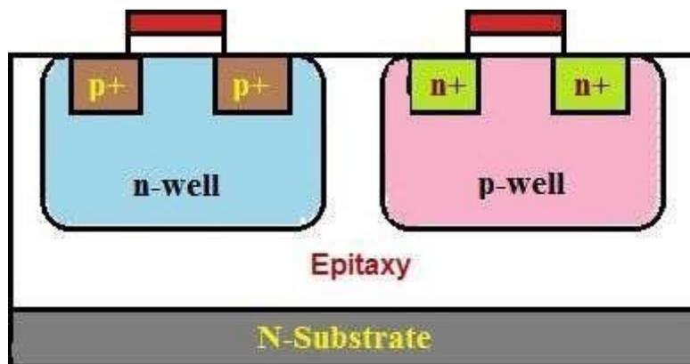
In this process, separate optimization of the **n-type and p-type transistors** will be provided. The independent optimization of  $V_t$ , body effect and gain of the P-devices, N-devices can be made possible with this process.
