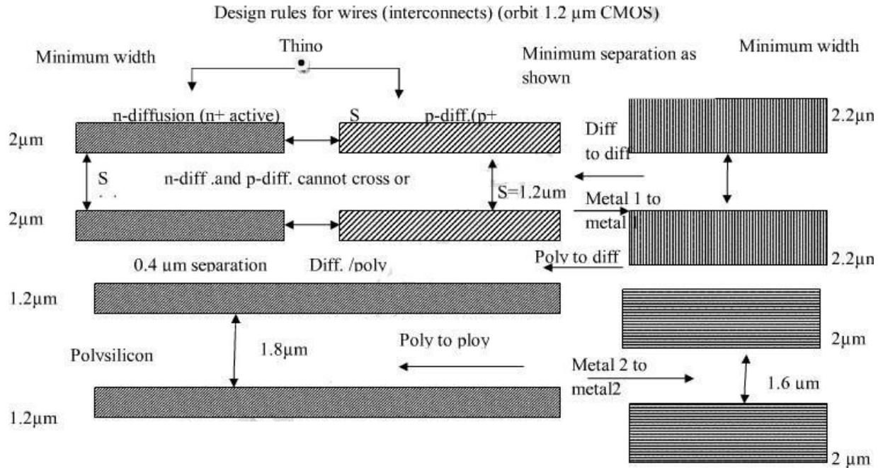
Avoid coincident edges where metal 1 and metal2 runs follow the same path for >25µm length (under lap metal 1 edges by 0.8 µm).
