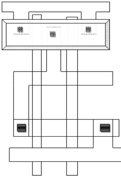
Metal mask for  $V_{DD}$ , GND and output connections
