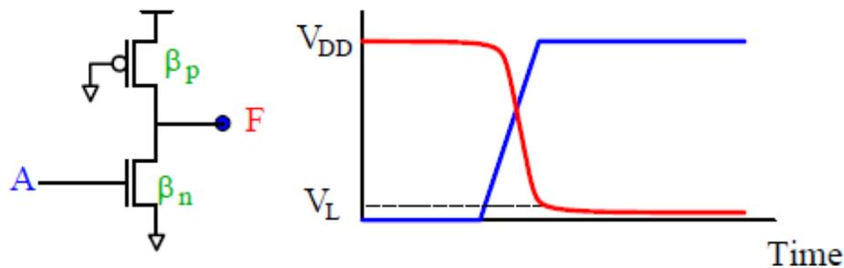
The inverter that uses a p-device pull-up or loads that has its gate permanently ground. An n-device pull-down or driver is driven with the input signal. This roughly equivalent to use of a depletion load is NMOS technology and is thus called '**Pseudo-NMOS**'. The circuit is used in a variety of CMOS **logic** circuits.
