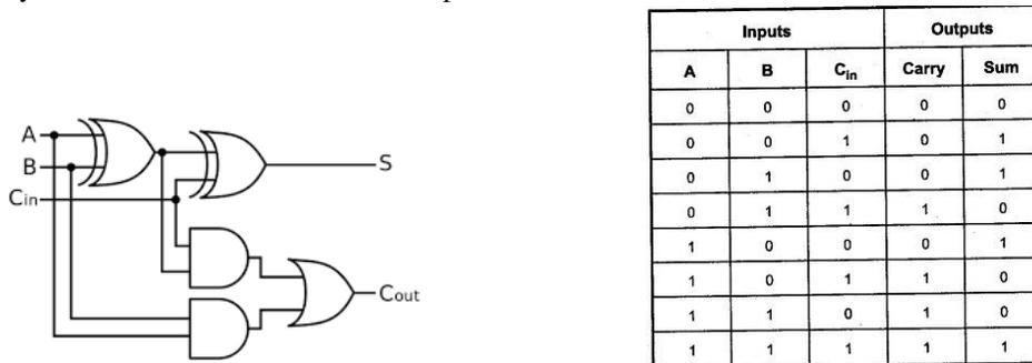
$N$ -bit adders take inputs  $\{A_N, \dots, A_1\}$ ,  $\{B_N, \dots, B_1\}$ , and carry-in  $C_{in}$ , and compute the sum  $\{S_N, \dots, S_1\}$  and the carry-out of the most significant bit  $C_{out}$ . They are called carry-propagate adders (CPAs) because the carry into each bit can influence the carry into all subsequent bits.
