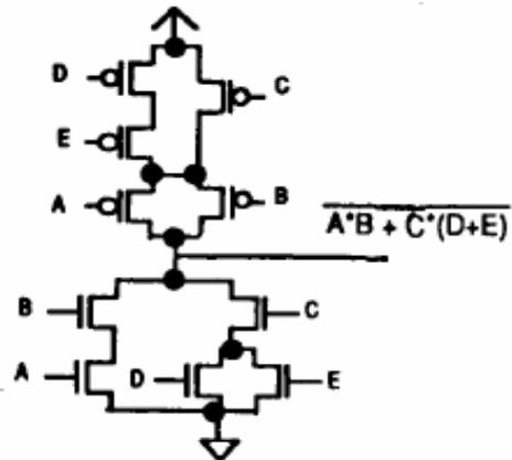
**Example Gate: COMPLEX CMOS GATE**
