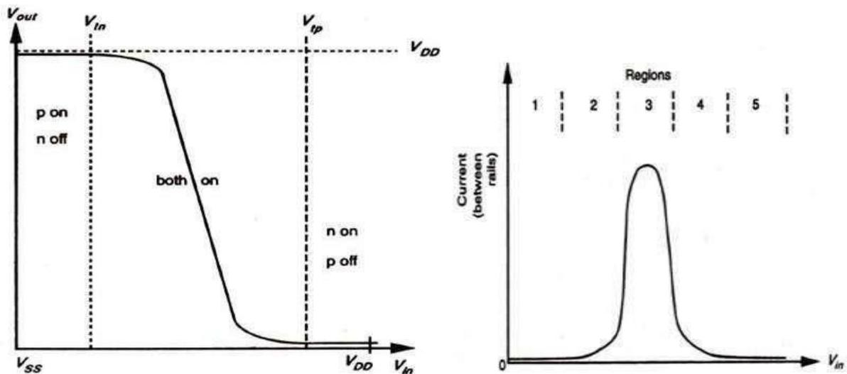
Hence the output voltage is logic 1. In region 5,  $V_{in} = \text{logic } 1$  and the n-transistor is fully on while the p-transistor is fully off. So, no current flows and logic 0 appears at the output.
