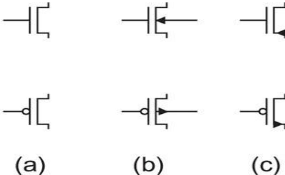
**FIG 2.1****MOS transistor symbols****ENHANCEMENT AND DEPLETION MODE MOS TRANSISTORS**
