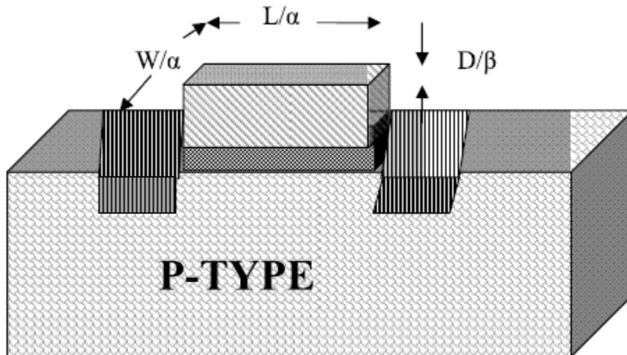
Two scaling factors  $1/\alpha, 1/\beta$  are used.  $1/\beta$  is chosen as the scaling factor for supply voltage  $V_{DD}$  and gate oxide thickness  $D$ , and  $1/\alpha$  is used for all other linear dimensions, both vertical and horizontal to chip surface.
