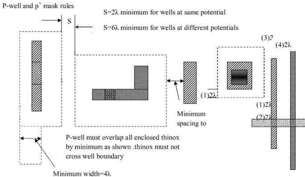
The CMOS rules are designed based on the extensions of the Mead and Conway concepts and also by excluding the butting and buried contacts the new rules for CMOS design are formed. These rules for CMOS design are implemented in the above diagrams.
