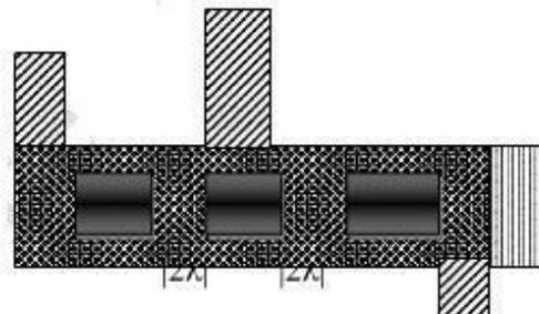
$2\lambda \times 2\lambda$  cut centered on  $4\lambda \times 4\lambda$  superimposed area of layers to be joined in all cases
