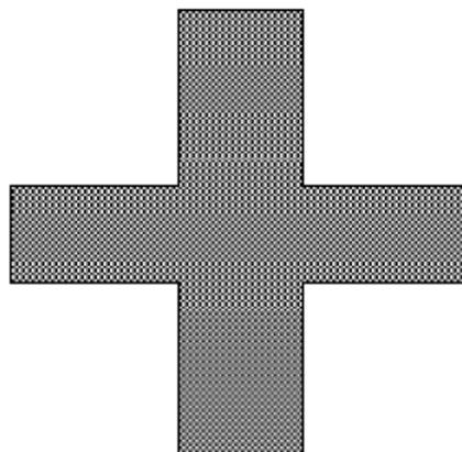
$$R = \text{square} \times R_s \frac{\text{Ohm}}{\text{square}} = R_s = 10^4 \text{ ohm.}$$
