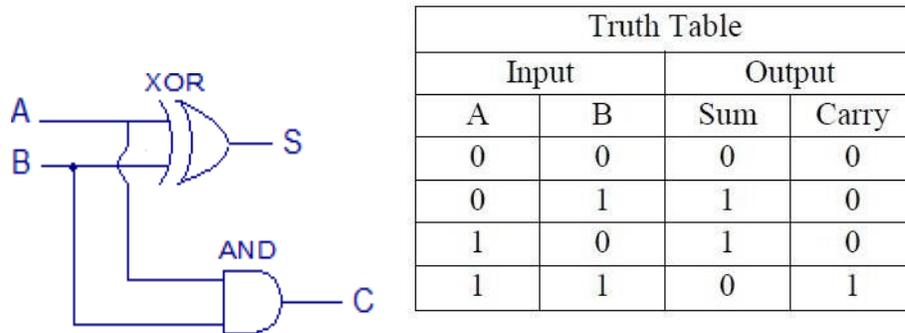
The carry-out is equivalent to a carry-in to the next more significant column of a multibit adder, so it can be described as having double the weight of the other bits. If multiple adders are to be cascaded, each must be able to receive the carry-in. Such a full adder has a third input called  $C$  or  $C_{in}$ .
