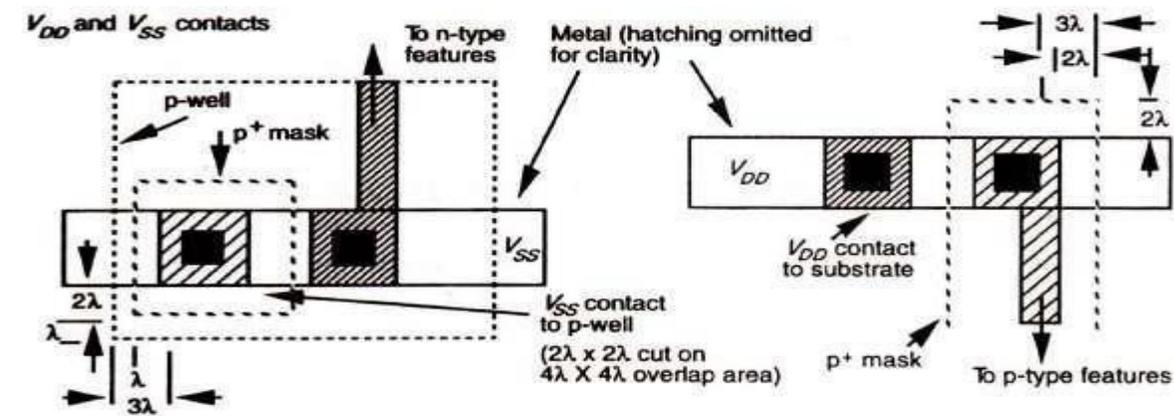
In the diagram above each of the arrangements can be merged into single split contacts.
