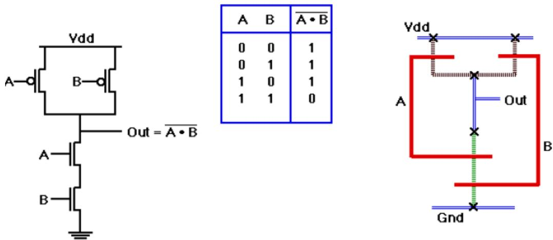
1. Pull-down: Connect to ground If A=1 AND B=1
