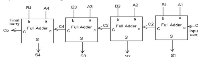
**Carry-Ripple Adder:** An N-bit adder can be constructed by cascading N full adders for N = 4. This is called a carry-ripple adder (or ripple-carry adder). The carry-out of bit i,  $C_i$ , is the carry-in to bit i + 1. This carry is said to have twice the weight of the sum  $S_i$ . The delay of the adder is set by the time for the carries to ripple through the N stages, so the  $t_{Cq} C_{out}$  delay should be minimized.
