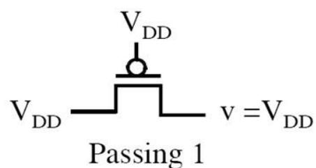
This is the reason that N-Channel transistors are used in the pull-down network and P-Channel in the pull-up network of a CMOS gate. Otherwise the noise margin would be significantly reduced.
