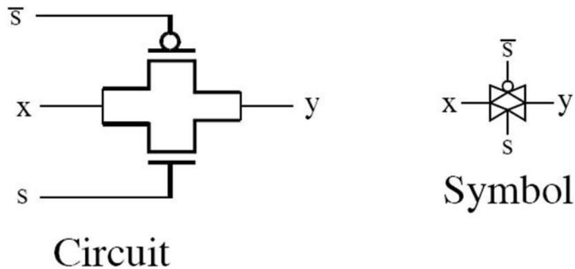
When  $s = 1$  the two transistors conduct and connect  $x$  and  $y$
