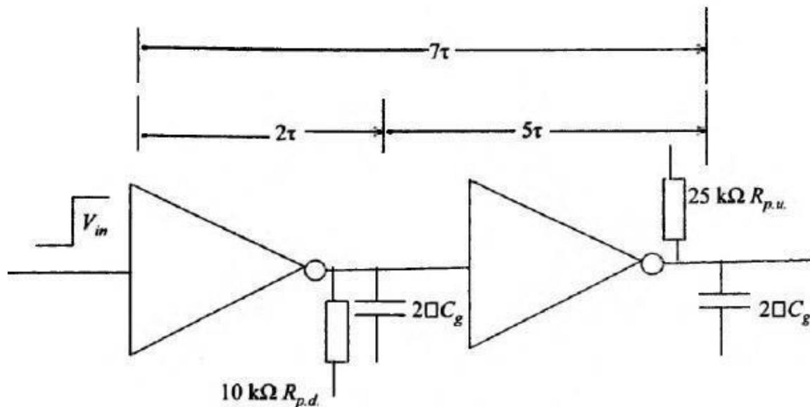
**Fig. 5.21** Minimum size CMOS inverter pair delay.
