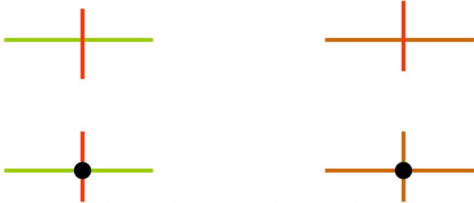
Note: If a contact is shown then it is ***not*** a transistor.
