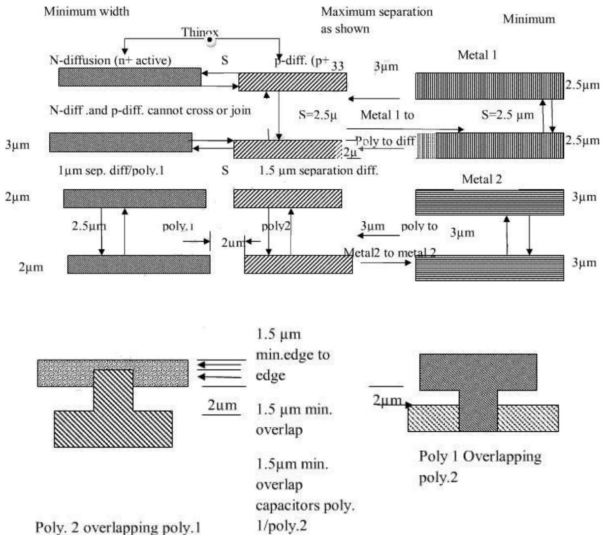
AVOID COINCIDENT EDGES WHERE METAL 1 AND METAL 2 RUNS FOLLOW THE SAME PATH FOR >25μm LENGTH (UNDER LAP METAL 1
