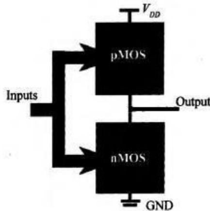
**Fig. 5.1** Standard configuration of a CMOS complementary gate.
