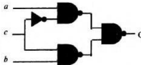
Fig. 5.9 (a) Standard 2-to-1 MUX design. (
