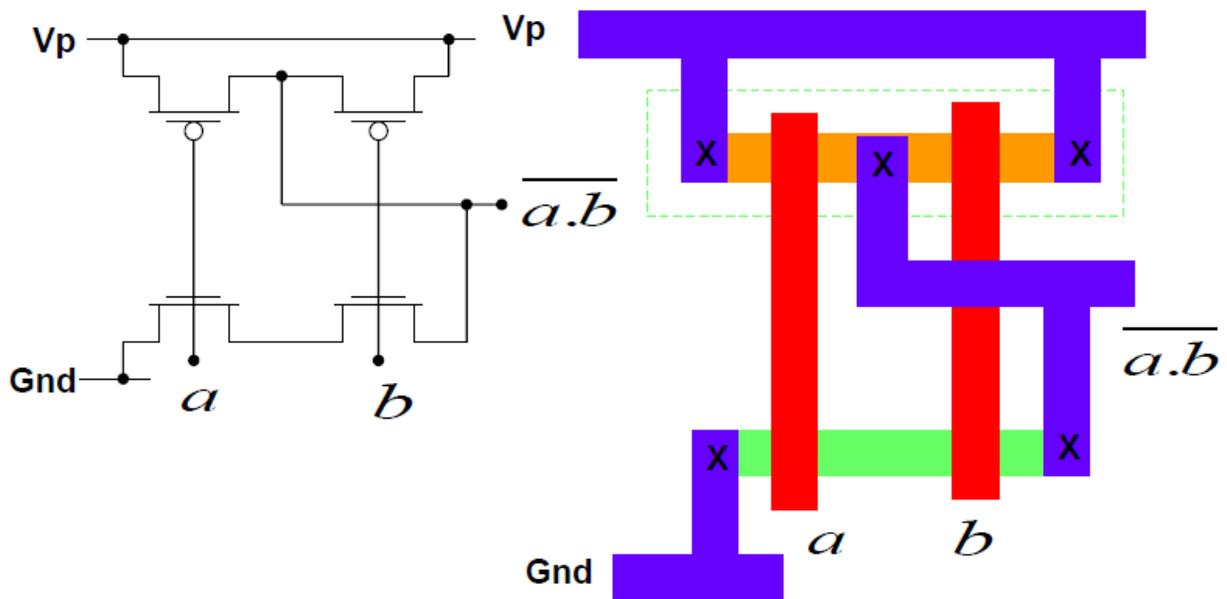
Layout & Stick Diagram of CMOS Inverter
